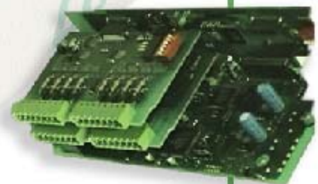
I/O Modules View
